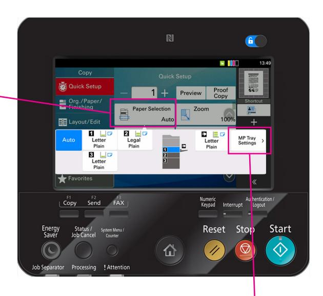
The MP tray (Multi-Purpose Tray) is on the right side of the machine and is used for copying or printing onto various media types.
