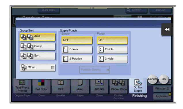
Finishing shows finishing options (i.e. sort/stapling/hole punch). (This will vary per machine depending on finisher configuration.)
